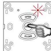
hold the remote control within 0.5mtr from receiver and press CLOSE button
